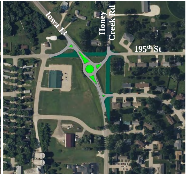
Figure 6: Single Roundabout Alternative
